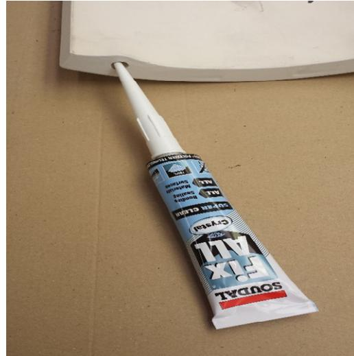
The holes are app. 2 cm deep and should be filled up app. 1/3 with adhesive as shown on the photo to the right.
